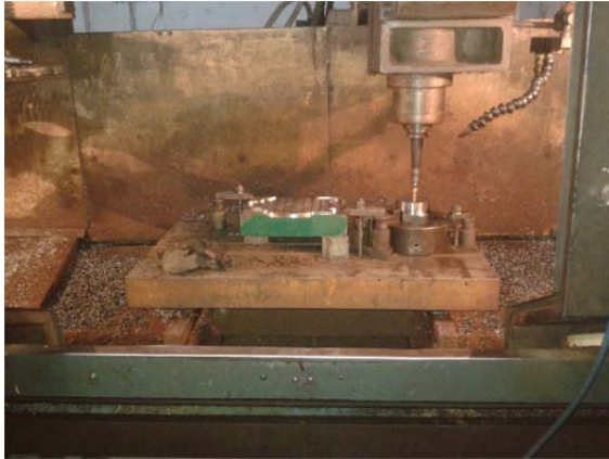
Fig. 2.1: Milling on VMC-640 manufactured by Jyoti CNC
